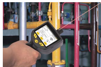
Leak detection from distance with the integrated laser pointer
